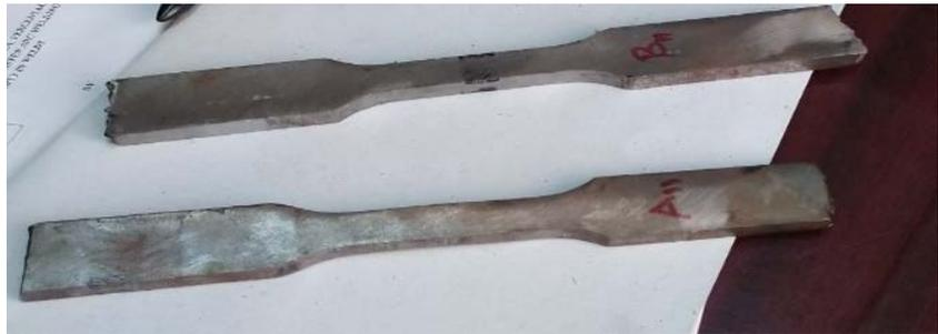
**Figure 5.** Dogbone specimen for A<sub>11</sub> and B<sub>11</sub>.
