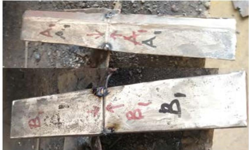
**Figure 4.** A<sub>11</sub> and B<sub>11</sub> tack welded specimen.
