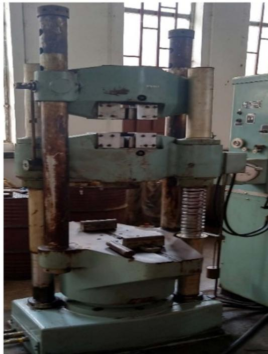
**Figure 6.** Tensile testing machine.
