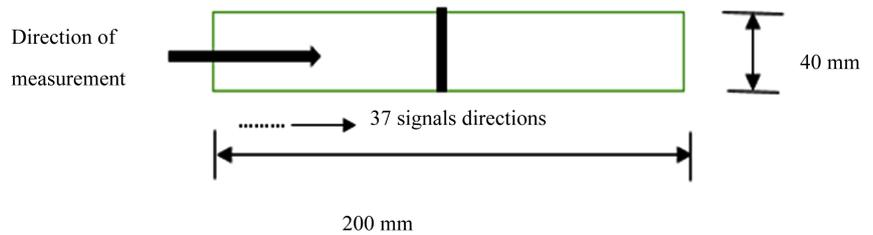
Figure 9. Direction of R.S Measurement on specimen.
