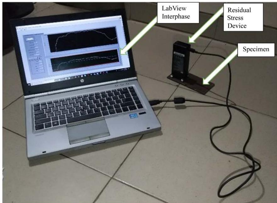
Figure 1. Magnetic measuring device.
