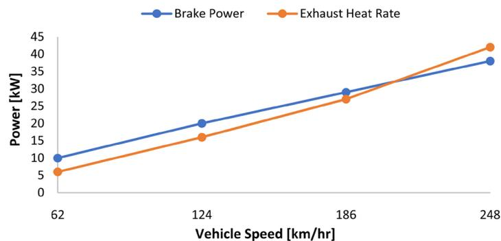
**Figure 4.** Engine brake power vs. power lost in exhaust.
