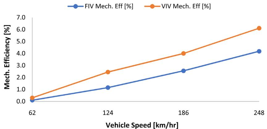
**Figure 6.** Mechanical efficiency due to ORC system.
