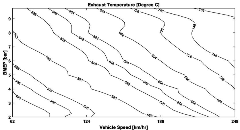
**Figure 2.** Exhaust temperature distribution.
