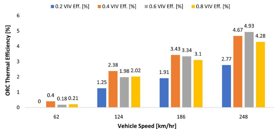
**Figure 9.** System efficiency achieved at VIV positions.
