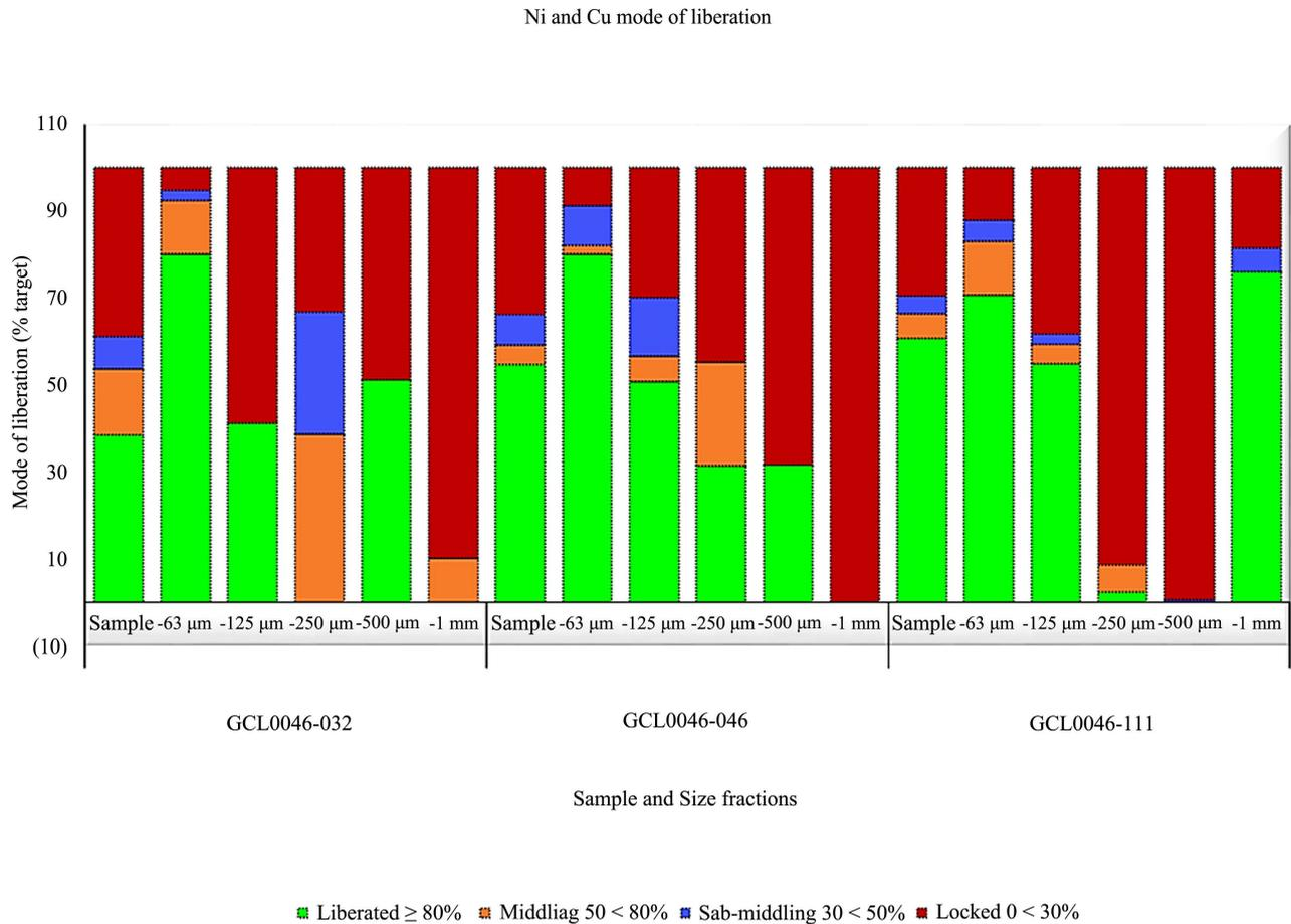
**Figure 11.** Ni and Cu-sulphides mode of liberation for from the waste rock samples across size fractions.
