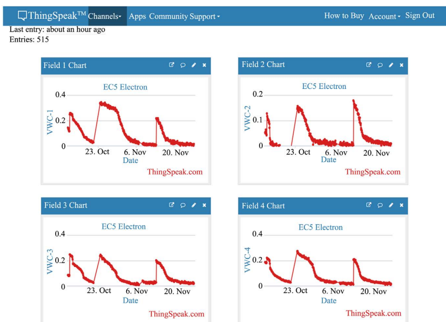
Figure 9. The Volumetric Water Content (VWC) of soil collected during 3 drying cycles in the laboratory using four Decagon EC-5 sensors.
