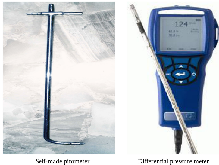
Figure 2. Physical image of the inspection device.
