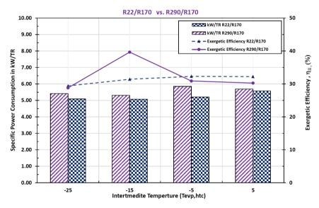
**Figure 12.** Specific power consumptions in kW/TR and exergetic efficiencies ( $\eta_{II}$ ) for cascade refrigeration cycles consist of two refrigerant pairs (R22/R170, and R290/R170) versus different intermediate temperature ( $T_{inter}$ ) –25°C, –15°C, –5°C, and +5°C.
