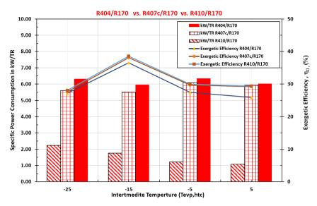
**Figure 11.** Specific power consumptions in kW/TR and Exergetic Efficiencies ( $\eta_{II}$ ) for cascade refrigeration cycles consist of three refrigerant pairs (R404/R170, R407c/R170, and R410/R170) versus different intermediate temperature ( $T_{inter}$ ) –25°C, –15°C, –5°C, and +5°C.
