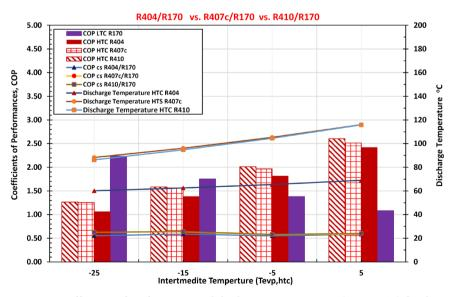
**Figure 8.** Coefficients of performance and discharges temperatures ( $T_6$  at HTC) for three refrigerant pairs (R404/R170, R407c/R170, and R410/R170) versus different intermediate temperature ( $T_{inter}$ ) –25°C, –15°C, –5°C, and +5°C.
