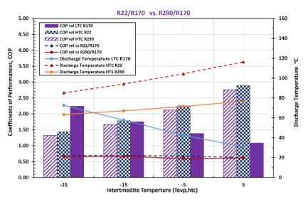
**Figure 9.** Coefficients of performance and discharges temperatures ( $T_2$  at LTC and  $T_6$  at HTC) for two refrigerant pairs (R22/R170, and R290/R170) versus different intermediate temperature ( $T_{inter}$ ) –25°C, –15°C, –5°C, and +5°C.
