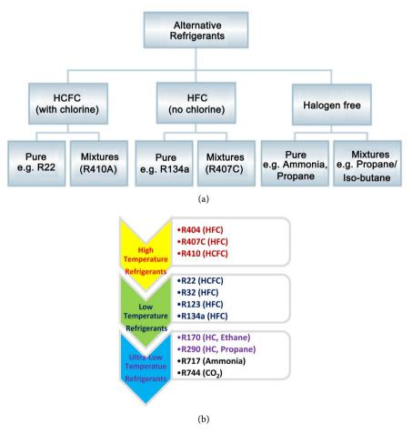
**Figure 6.** Refrigerant classification based on their chemical composition, and on their working temperature ranges. (a) based on their chemical composition, (b) based on their classification on their working temperature ranges, high, low, and ultra-low temperature ranges, which are numerically investigated in the current research.
