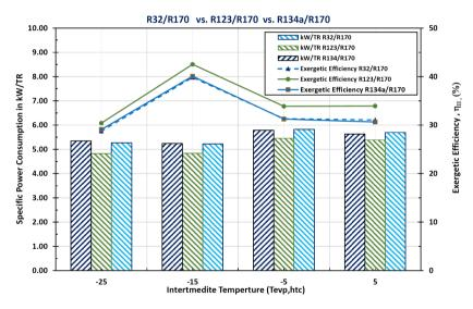
**Figure 10.** Specific power consumptions in kW/TR and Exergetic Efficiencies ( $\eta_{II}$ ) for cascade refrigeration cycles consist of three refrigerant pairs (R32/R170, R123/R170 and R134a/R170) versus different intermediate temperature ( $T_{inter}$ ) –25°C, –15°C, –5°C, and +5°C.
