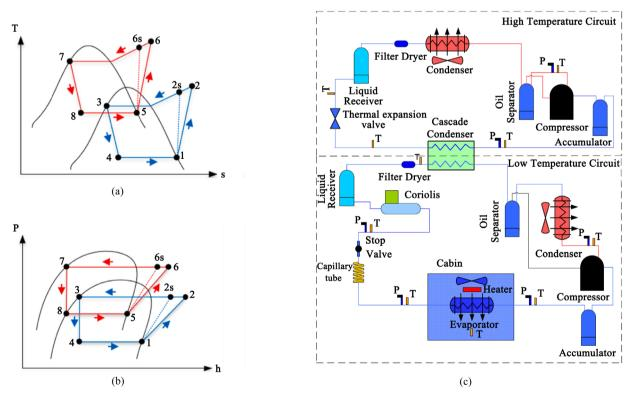
**Figure 5.** Cascade refrigeration cycle proposed as innovative refrigeration system for COVID-19 vaccines transportation and storage. (a), (b) CRS presented on T-s diagram and on p-h diagram, respectively, presented by Aktemur *et al.* [18], and (c) Line diagram for CRS with LTC and HTC, presented by Alhamid *et al.* [36].
