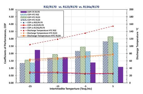
**Figure 7.** Coefficients of performance and discharges temperatures ( $T_6$  at HTC) for three refrigerant pairs (R32/R170, R123/R170 and R134a/R170) versus different intermediate temperature ( $T_{inter}$ ) –25°C, –15°C, –5°C, and +5°C.
