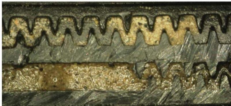
**Figure 1.** Clogging of emitters in practical application.
