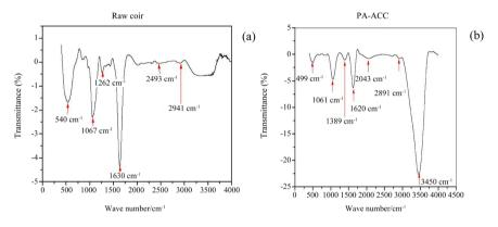
Figure 2. FT-IR analysis of (a) raw coconut coir and (b) (PA-ACC) activated coconut coir based carbon.
