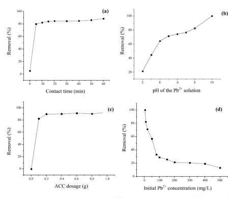
**Figure 5.** Lead(II) removal percentages at different (a) contact times (min) (b) pH levels and (c) ACC dosages (g) and (d) initial lead(II) concentrations (ppm).
