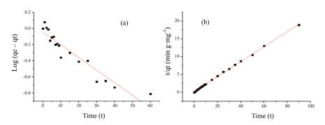
**Figure 6.** Adsorption kinetic study of Pb<sup>2+</sup> adsorption on phosphoric activated ACC (a) pseudo first order kinetic model (b) pseudo second order kinetic model.
