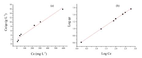
**Figure 7.** Adsorption isotherms study of Pb<sup>2+</sup> adsorption on phosphoric activated ACC (a) Langmuir isotherm model (b) Freundlich isotherm model.
