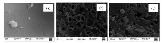
Figure 3. SEM images of (a) raw coconut coir and (b) ACC.
