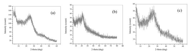
Figure 1. XRD defractogram of (a) raw coconut coir, (b) phosphoric activated ACC (PA-ACC) and (c) lead adsorbed PA-ACC.
