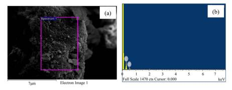
**Figure 4.** (a) Focused area on the surface and (b) EDX spectrum of the ACC surface and (b) EDX spectrum of the ACC.
