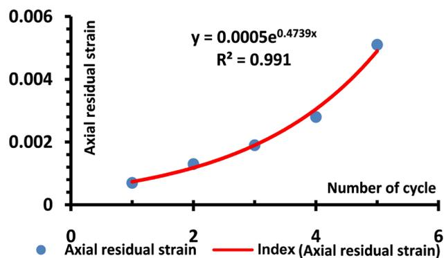
**Figure 11.** Residual strain relation according to the number of cycle.
