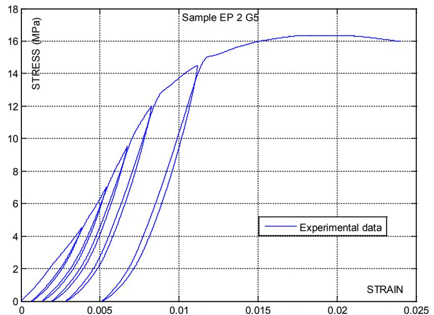
Figure 4. stress-strain curve of a cyclic compression test.
