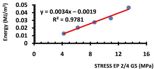
Figure 7. Energy curve as function of the strain level per cycle.
