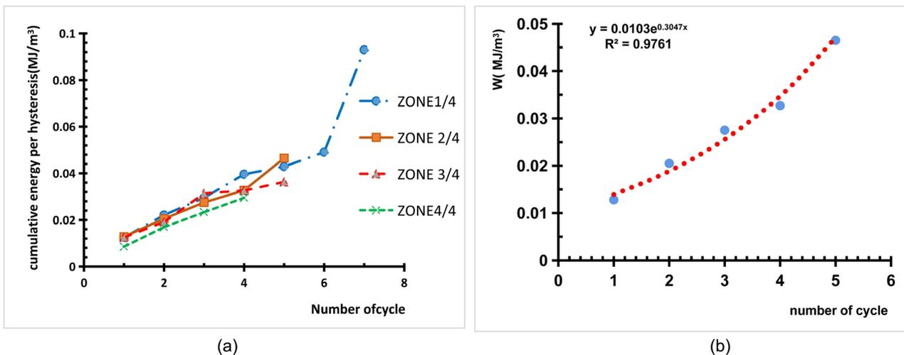
Figure 8. cumulative energy curves by hysteresis as a function of the number of cycles.
