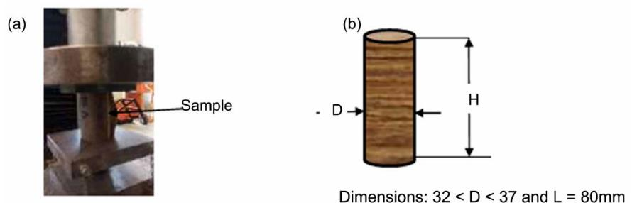
Figure 2. Image of test sample on compression (a) and dimensions of sample (b).
