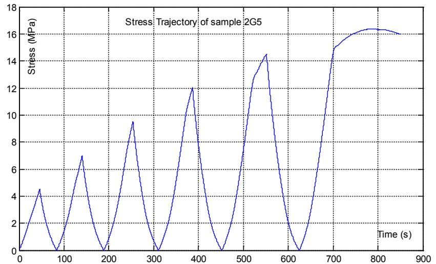
Figure 3. Stress trajectory following charge-discharge.
