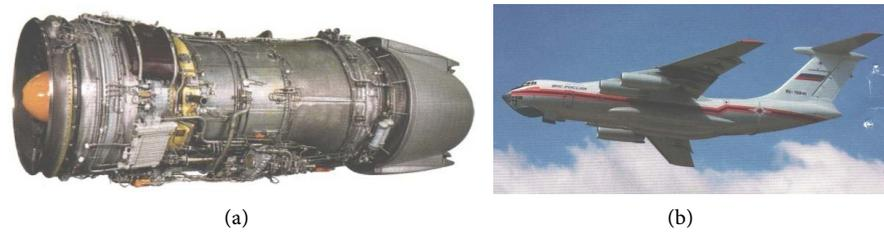
**Figure 16.** Gas turbine engine D-30KP-2, with a thrust of 12,000 kg (a); D-30KP-2 on an IL-76 aircraft, with a carrying capacity of 50 tons (b).
