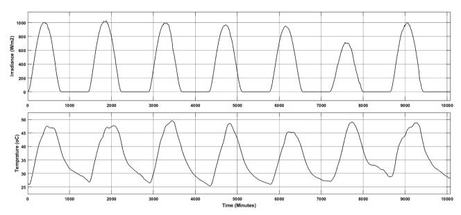
Figure 11. Irradiance and temperature during 1st week of April.
