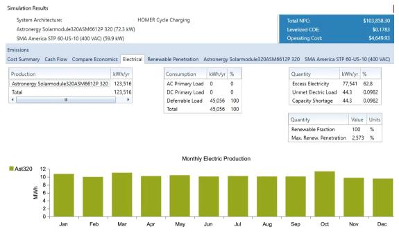
Figure 19. Simulation details for proposed system with water tank.
