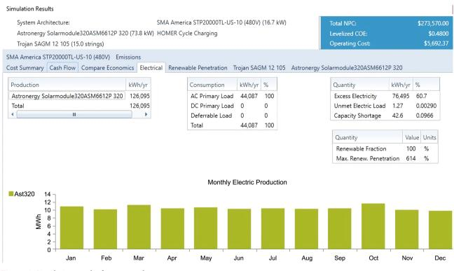
Figure 6. Simulation results for proposed system.
