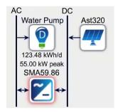
Figure 18. Proposed solar water pumping system with water tank.
