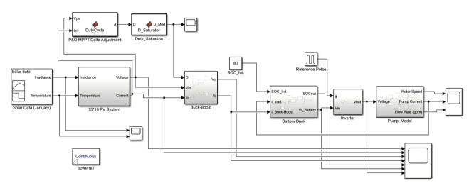
Figure 10. Dynamic model of proposed solar water pumping system with battery bank.
