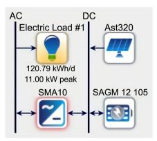
Figure 5. Proposed solar water pumping system with a battery bank.
