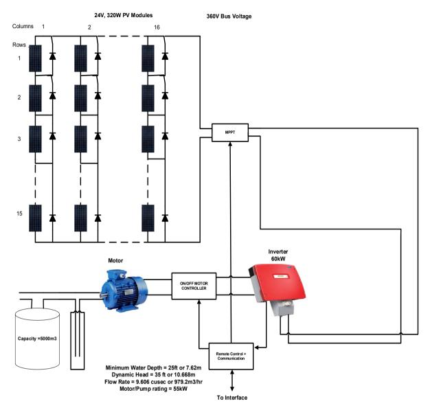
Figure 20. Proposed solar water pumping system with water tank.
