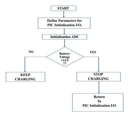
Figure 2. Charging flowchart for PIC programming.
