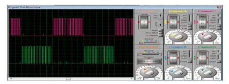
Figure 9. PWM signals generated by microcontroller.
