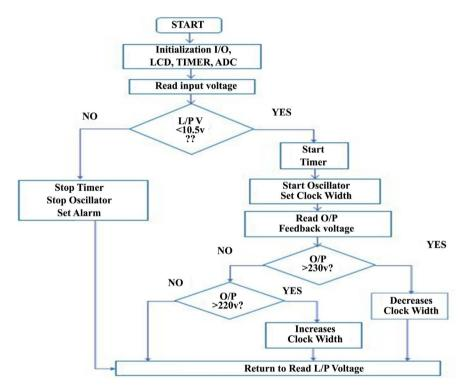
Figure 4. Flowchart of inverter for PIC programming.
