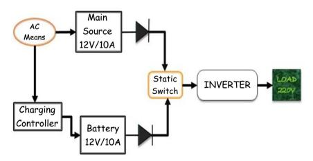
Figure 1. Block diagram of DSP control UPS system.
