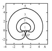
**Figure 1.** Stages (2, 3, 4) of formation of the dislocation loop from the ED (1). The axis *x* is directed along the initial position of the ED, the axis *y* determines the deviation of the ED from the equilibrium position (*x* and *y* are measured in units of the lattice spacing *b*).
