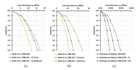
**Figure 2.** Effect of over consolidation ratio on the cone tip resistance performance line. (a) Effect of sand type on the value of  $q_{cs}$  (b) Variation of OCR from [3]; (c) Variation of OCR from [20].
