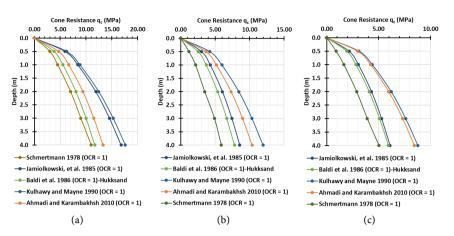
**Figure 4.**  $q_c$  profile for Normally consolidated sands. (a)  $D_r = 85\%$ ; (b)  $D_r = 70\%$ ; (c)  $D_r = 60\%$ .
