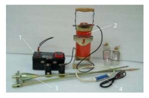
Figure 1. Radon measuring device diagram.
