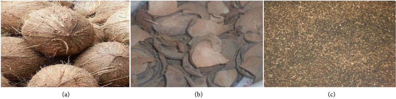
**Figure 2.** Process for obtaining coconut particles. (a) Coconut; (b) Coconut shells; (c) Crushed and sifted hulls.
