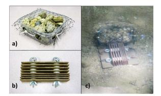
**Figure 2.** Deployed samplers: tray and low-profile Hester-Dendy. (a) Assembled gravel-filled tray; (b) Assembled modified Hester-Dendy (MHD); (c) Gravel tray and Hester-Dendy deployed in a pool on Congress Run.
