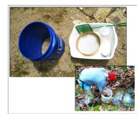
Figure 3. Bucket grab sampling method, showing equipment and sampling being performed.
