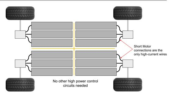
Figure 5. Distributed power electronics EV drivetrain.
