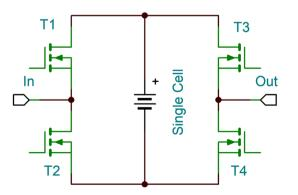
Figure 2. single cell MMC module.
