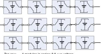
Top row: 4 modules in series; full +ve voltage Middle row: 4 modules in series; full -ve voltage Bottom row: 2 modules in series 2 short circuit, half +ve voltage
