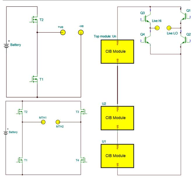
Figure 3. Module options, top left single I-bridge, the full cascade CIB is shown right in a section configuration. Bottom left H-bridge.
