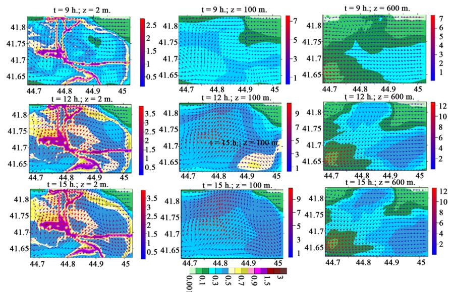
**Figure 3.** Wind velocity (m/sec) and dust concentration (MAC) distribution, when  $t = 9, 12$  and  $15$  h at  $2, 100$  and  $600$  m height over ground.
