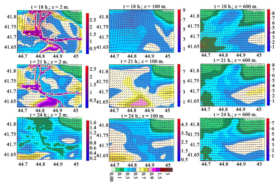
**Figure 4.** Wind velocity (m/sec) and dust concentration (MAC) distribution, when  $t = 18, 21$  and 24 h at 2, 100 and 600 m height over ground.
