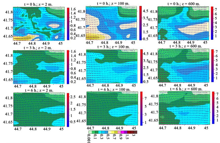
**Figure 2.** Wind velocity (m/sec) and dust concentration (MAC) distribution, when  $t = 0, 3$  and  $6$  h at  $2, 100$  and  $600$  m height over ground.
