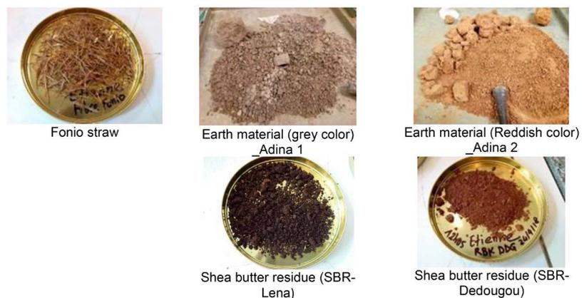
**Figure 1.** Earth material and stabilizers specimens.
