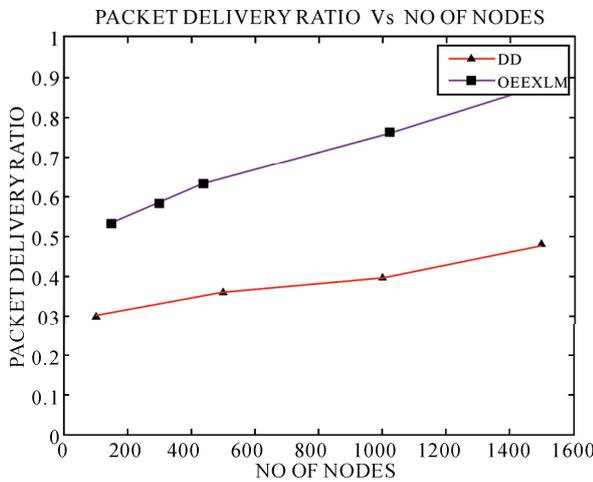
Figure 11. Packet delivery ratio vs number of nodes.
