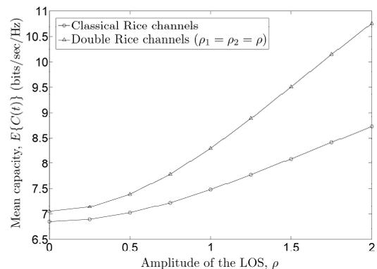
Figure 5. The mean capacity  $E\{C(t)\}$  of classical Rice and double Rice channels.
