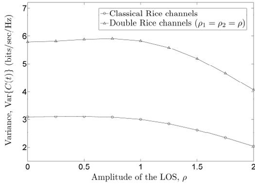
Figure 6. The variance  $\text{Var}\{C(t)\}$  of the capacity of classical Rice and double Rice channels.
