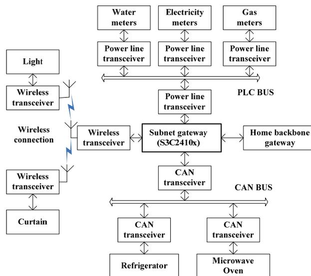
Figure 2. The typical structure of home control subnet.
