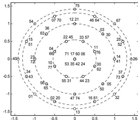
Figure 3. Signal constellation of superposition 8PSK modulation.
