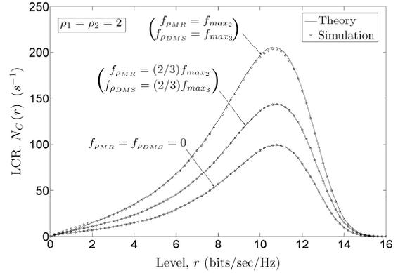
Figure 9. The LCR  $N_C(r)$  of the capacity of double Rice channels.
