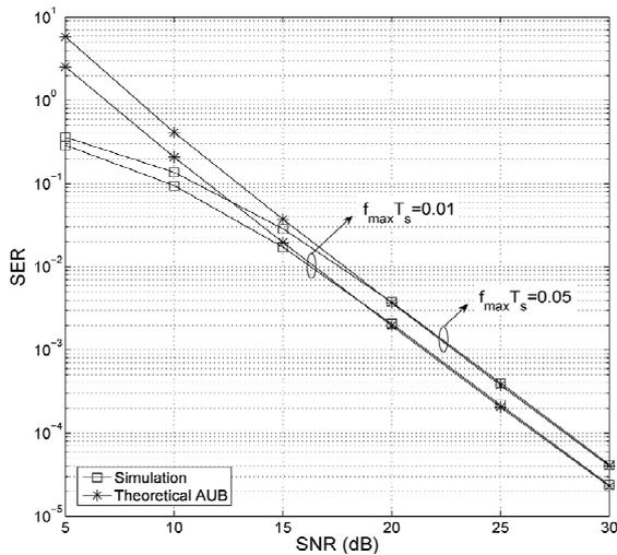
Figure 2. Comparison of the theoretical AUB and simulation results of the SER for the AF cooperative communication systems with various values of the normalized maximum Doppler frequency  $f_{\max} T_s$ .
