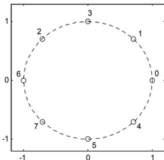
Figure 2. Signal constellation of 8PSK modulation.
