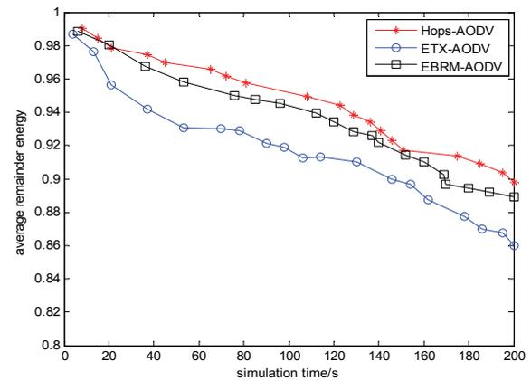
**Figure 4. The relationship between remainder energy and time.**
