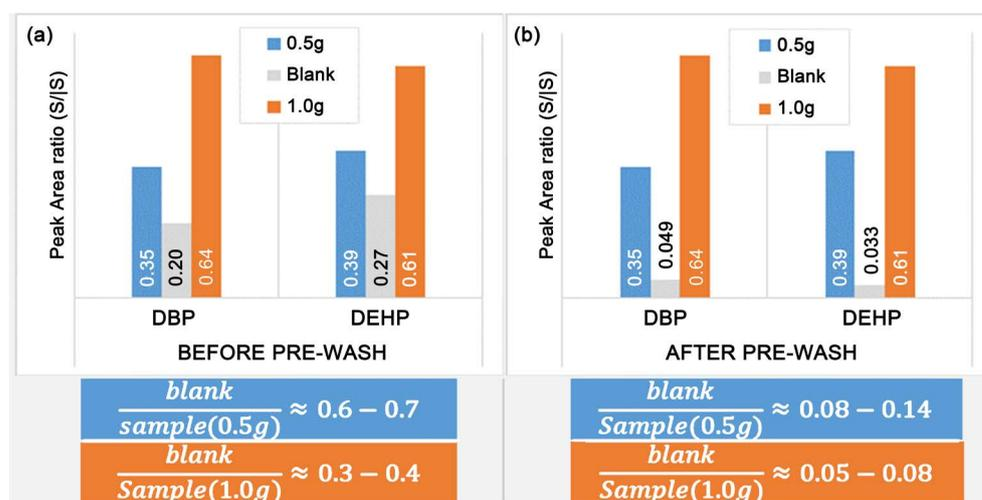
**Figure 2.** Reducing contributions to PAE contamination along the procedure. (a) Effect of sample amount on the ratio of PAEs extracted from the blank (diatomaceous earth extracted by hexane), to PAEs derived from the sample; (b) Impact of diatomaceous earth prewash procedure on this ratio.
