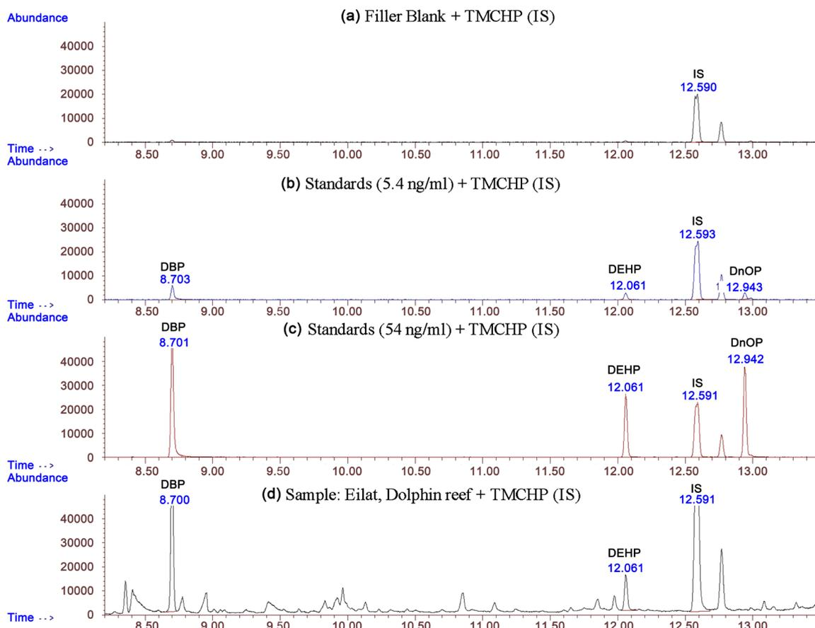
**Figure 3.** GC-MS chromatograms. (a) Filler blank sample + IS; (b) PAE standards (5.4 ng/mL) + IS; (c) PAE standards (54 ng/mL) + IS; (d) Chromatogram of a representative sample (Eilat, Dolphin Reef) + IS.
