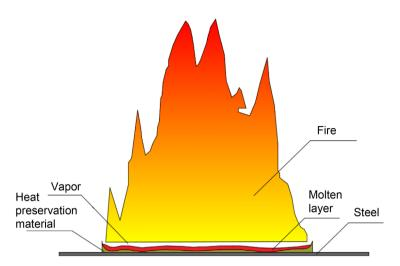
Figure 1. Schematic diagram of thermal insulation material combustion.
