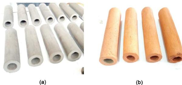
**Figure 12.** Tubular ceramic supports, (a) before sintering and (b) after sintering.
