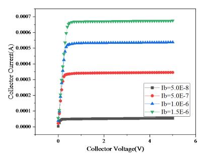
**Figure 3.** Output characteristics of the device when the Ge component of the base region is trapezoidal.
