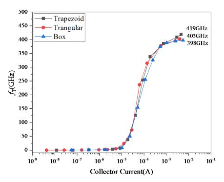
**Figure 5.**  $f_{\rm T}$  versus  $I_{\rm c}$  curve for Ge component SOI SiGe HBT in different base regions.
