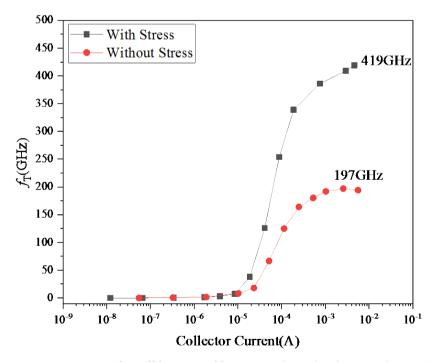
**Figure 7.** Comparison of cutoff frequency  $f_{\rm T}$  between traditional and proposed SOI SiGe HBT.
