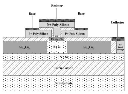
Figure 1. Structure of proposed SOI SiGe HBT device.
