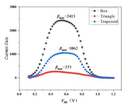
**Figure 2.** Relationship between  $\beta_{\text{max}}$  and  $V_{BE}$  with three different distributions of Ge components in the base.
