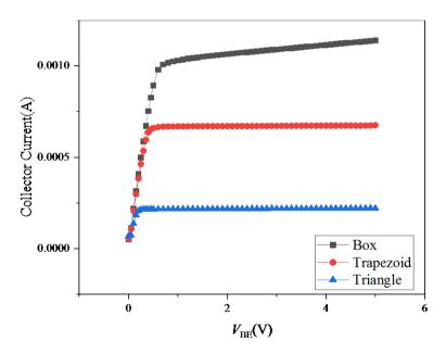
**Figure 4.** *I*-*V* characteristics of the three base Ge component distributions @  $I_{\rm B}$  = 1.5  $\mu$ A.
