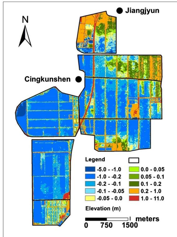
**Figure 5.** Classification of the terrain elevation map of the Cigu salt pan using a DEM and the ArcGIS 10.3 Reclassify tool.
