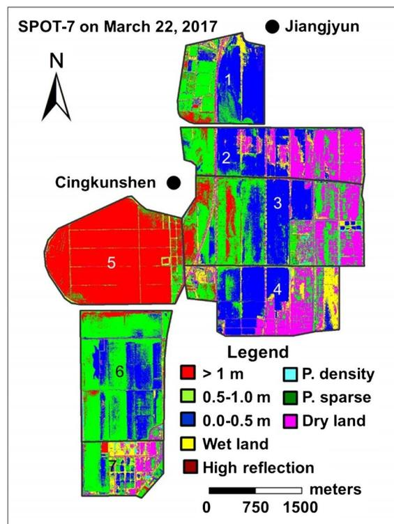
**Figure 7.** Classification of the water depth maps of Cigu salt pan from satellite images obtained using SPOT 7 on March 22, 2017, using ENVI 4.8 software.
