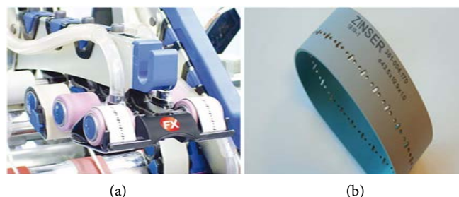
Figure 7. (a) The centrepiece of Zinser Impact FX & (b) Compacting apron [22].
