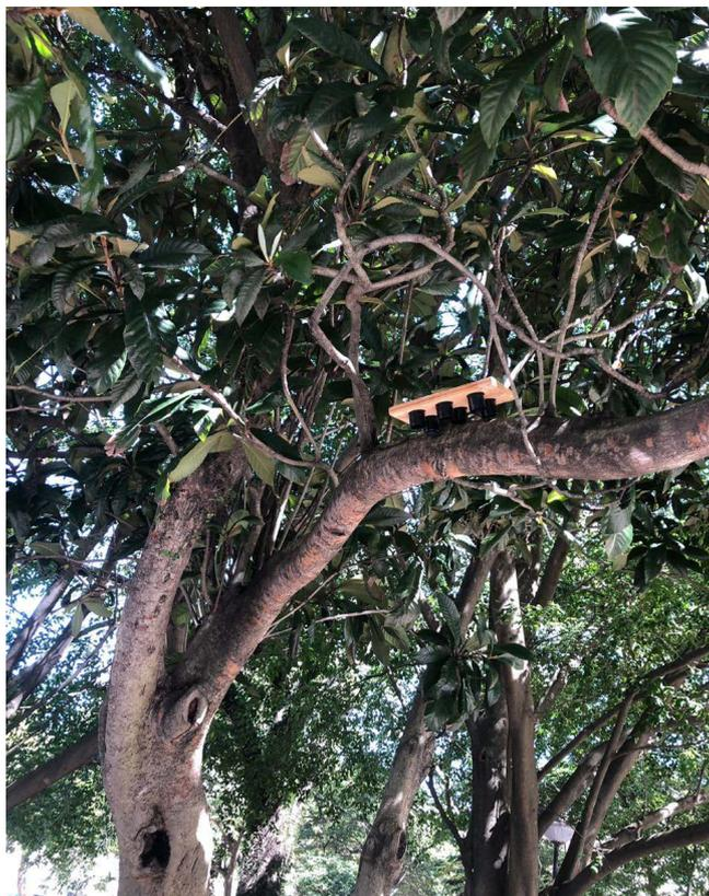
**Figure 2.** Filters of  $\text{NO}_2$  and  $\text{O}_3$  installed in park trees for monitoring sampling.
