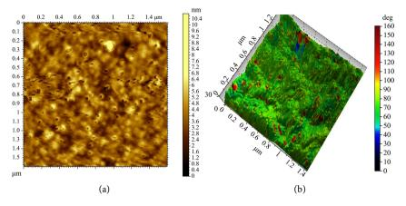
**Figure 2.** Nano-Chs BM with stabilizer + UZD: Dimensions of nano-Chs-P: length—120 nm, width—7 nm.
