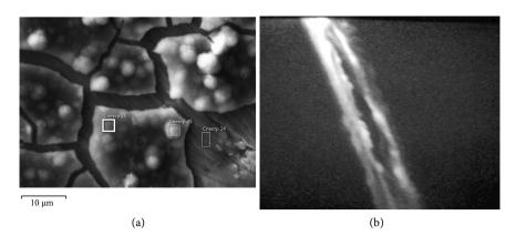
**Figure 3.** Chs-TCF coating image on a titanium plate, scale-10 microns. (a) CHS-Ca/P on a titanium plate, scale-10  $\mu$ m; (b) SEM-image coating of the end of the plate: the outer layer of Ca<sub>3</sub>(PO<sub>4</sub>)<sub>2</sub>, the inner (dark) layer of chitosan.
