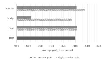
**Figure 6.** Packets per second for large packet transmission between different physical hosts.
