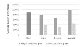
**Figure 5.** Packets per second for small packet transmission between different containers in the same physical host.
