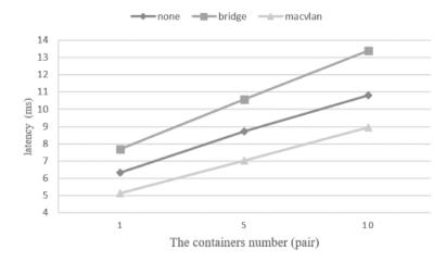
**Figure 8.** Large packet transmission latency between different containers in the same physical host.
