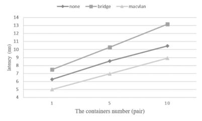
**Figure 9.** Small packet transmission latency between different containers in the same physical host.
