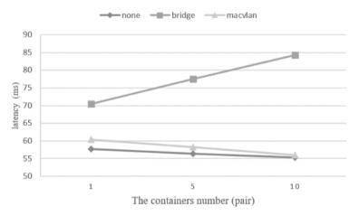
Figure 11. The latency of small packet transmission between different hosts.
