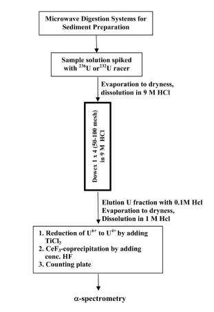
Figure 2. Schematic representation of the radiochemical separation of uranium.
