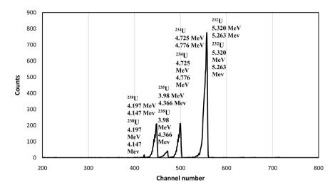
Figure 3. Spectrum result from Alpha spectrometry Using U-232 as a tracer for (WA5).
