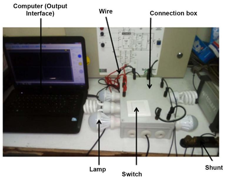
**Figure 2.** Harmonic spectrum experimental setup.
