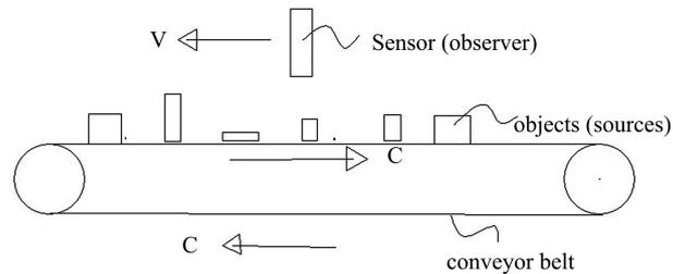
**Figure 2.** Sketch of a Conveyor Belt with a Doppler Shift.
