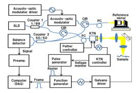
**Figure 1.** High-speed TD en face OCT system configuration. CIR: Circulator; PC: Polarization controller; DAQ: Data acquisition system.
