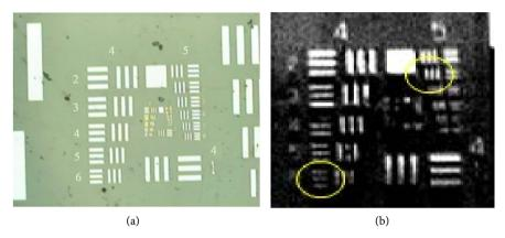
Figure 4. En face image of test chart (USAF 1951). (a) Photograph of test chart; (b) En face image of test chart.
