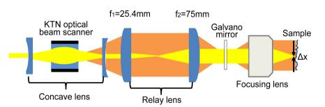
Figure 3. Beam propagation and optical arrangement of the sample arm.
