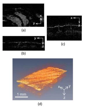
**Figure 6.** High-speed en face OCT images of human fingerprint. (a) En face OCT image of x-y plane; (b) OCT image of the y-z plane; (c) OCT image of x-z plane; (d) Constructed 3D-OCT.
