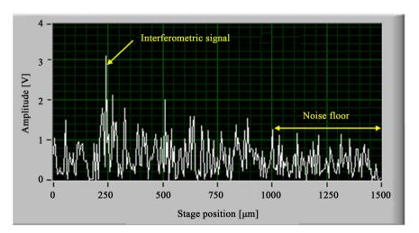
Figure 5. The measured signal-to-noise ratio (SNR) of the en face OCT system.
