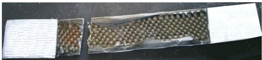
Figure SI-9. Failure mode type AGB (Angled Gage Bottom) of the specimen tested.
