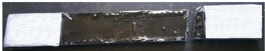
Figure SI-4. Failure mode type AGT (Angled Gage Top) of the specimen tested.
