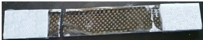
Figure SI-10. Failure mode type LGB (Lateral Gage Bottom) of the specimen tested.
