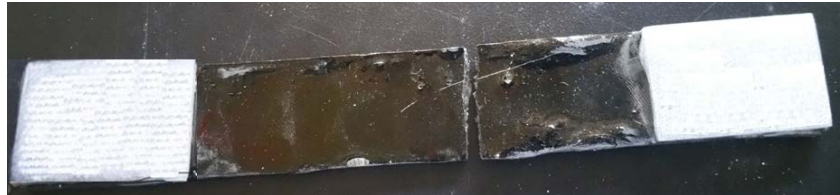
Figure SI-7. Failure mode type LGM (Lateral Gage Middle) of the specimen tested.
