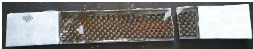
Figure SI-8. Failure mode type LGT (Lateral Gage Top) of the specimen tested.
