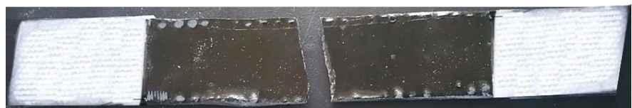
Figure SI-5. Failure mode type AGM (Angled Gage Middle) of the tested specimen.
