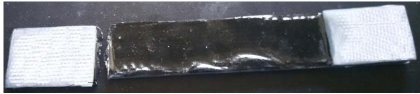
Figure SI-6. Failure mode type LAB (Lateral At grip/tab Bottom) of the specimen tested.
