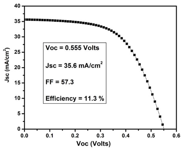
**Figure 3.** The 200 nm Cu/800nm Al metal sandwich grid pattern based CIGS solar cell current-voltage (I-V) output photo conversion efficiency curve.
