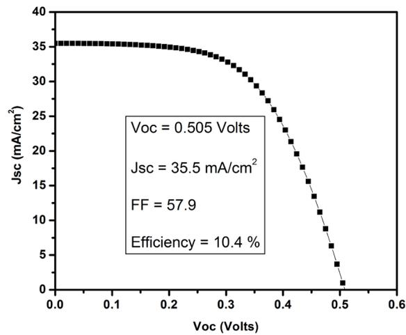
**Figure 2.** The 1  $\mu\text{m}$  Al metal grid pattern based CIGS solar cell current-voltage (I-V) output photo conversion efficiency curve.
