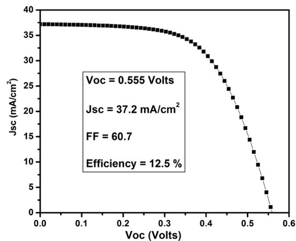
**Figure 4.** The 200 nm Al/800nm Cu metal sandwich grid pattern based CIGS solar cell current-voltage (I-V) measurement output and photo conversion efficiency curve.
