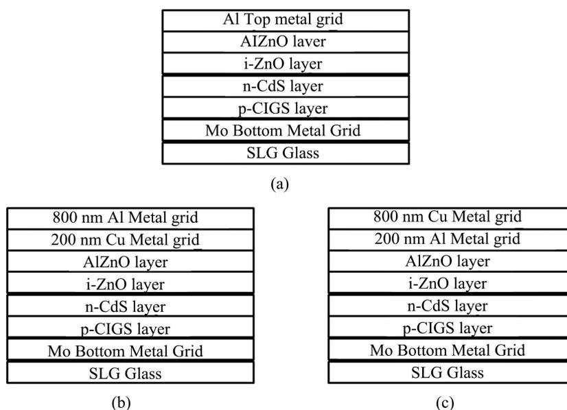
**Figure 1.** (a) (b) (c) the complete CIGS solar cell structure with various top grid metal sandwich patterns.
