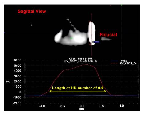
**Figure 3.** Quantification of gold fiducial length on the cone-beam CT image dataset by using the width of Hounsfield unit (HU) number of zero along the track of fiducial motion. Window/level setting for abdomen was used in the Eclipse treatment planning software.
