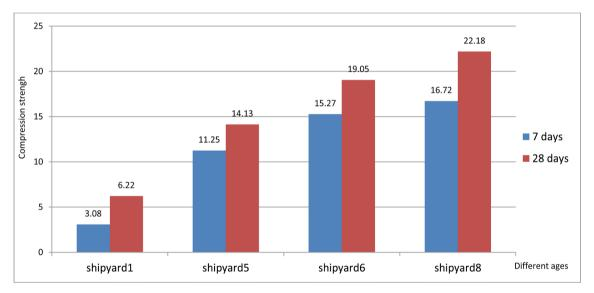
Figure 6. Resistance results of concretes to compression (two measures).
