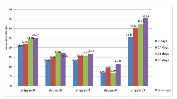
Figure 5. Resistance results of concretes to compression (four measures).
