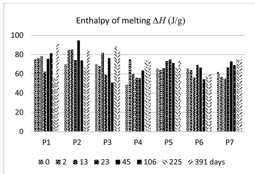
**Figure 2.** Dependence of the enthalpy of melting on the ageing time for the seven specimens P1 to P7.
