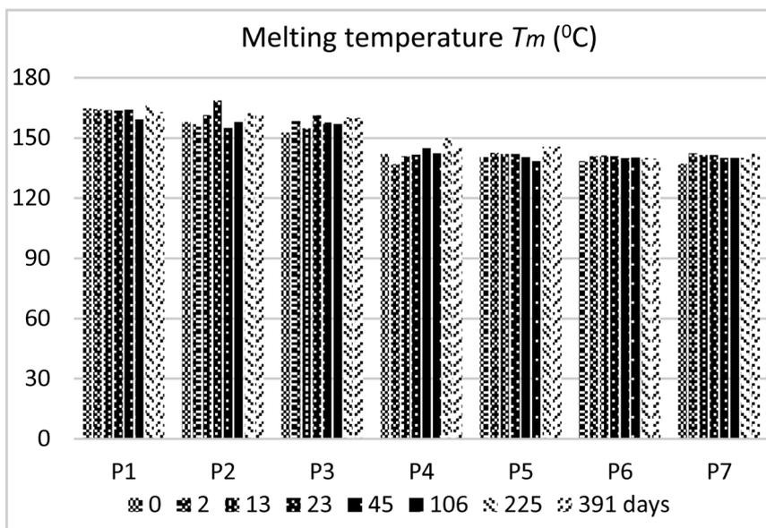
Figure 4. Dependence of the melting temperature on the ageing time for the seven specimens P1 to P7.
