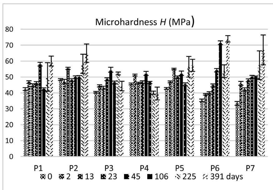
**Figure 1.** Dependence of the microhardness on the ageing time for the seven specimens P1 to P7.
