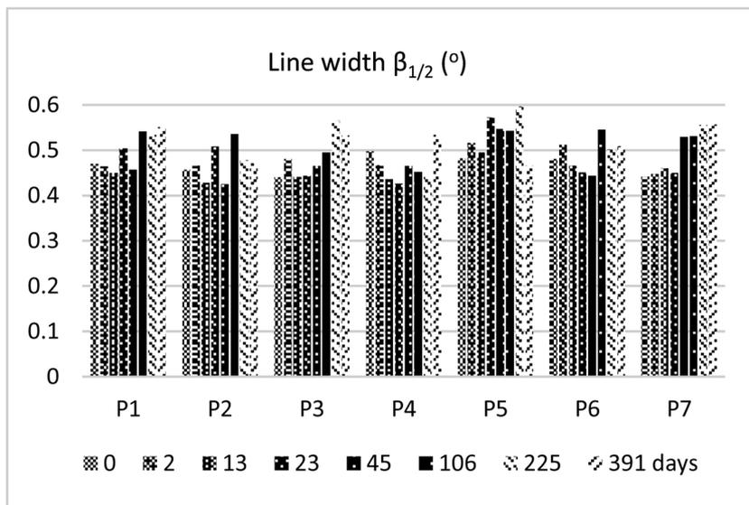
Figure 3. Dependence of the line 040 width on the ageing time for the seven specimens P1 to P7.
