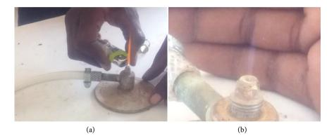
**Figure 4.** Flammability test set-up. (a) Propagation of the flame; (b) Complete combustion of the biogas.
