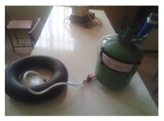
Figure 3. Generation of biogas from food waste.
