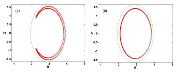
**Figure 2.** (a) The electrostatic field E is zero, particle is trapped; (b) The electrostatic field E is -35 kv/m, particle is turned to be circulating which is called as de-trapping. Ion energy is 60 kev, pitch angle 151°.
