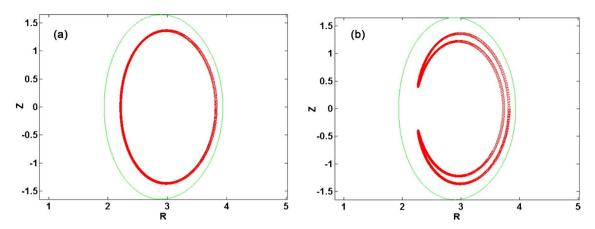
**Figure 1.** (a) The electrostatic field E is zero, particle is circulating; (b) The electrostatic field E is 35 kv/m, particle is trapped. Ion energy is 60 kev, pitch angle is 72°.
