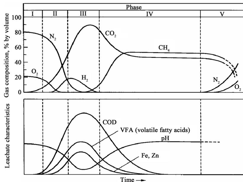
**Figure 12.** Schematic presentation of biogas production stages. Source: "Integrated Solid Waste Management" G. Tchobanoglous, H. Theisen, S. Vigil [4].
