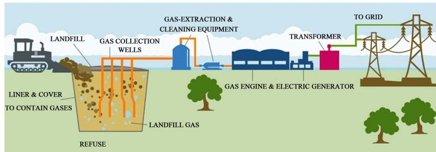
**Figure 4.** Process of converting biogas to electricity [3].
