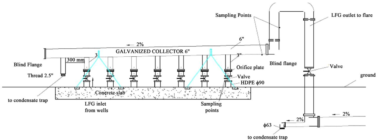
**Figure 9.** Typical drawing of manifold [1].
