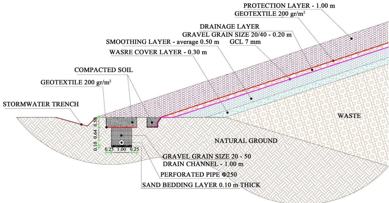
Figure 5. Layer of final capping [1].
