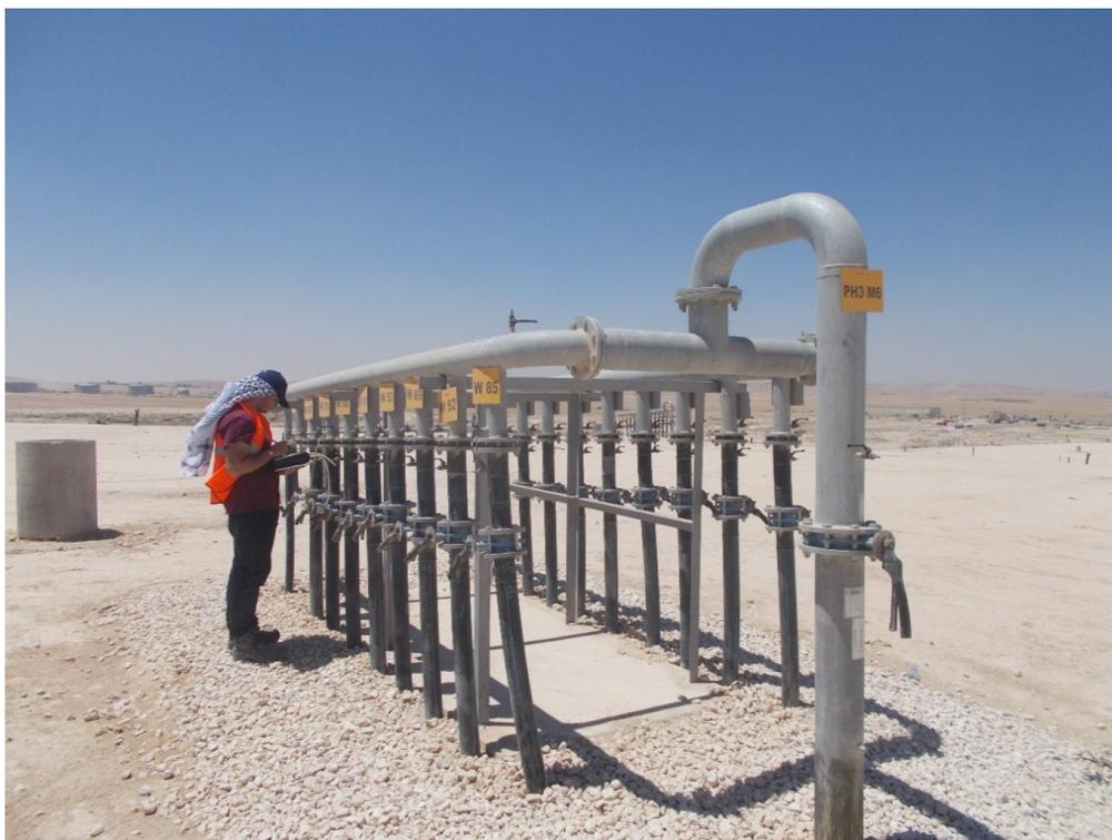
Figure 8. Measurement of gas concentration in the manifolds.
