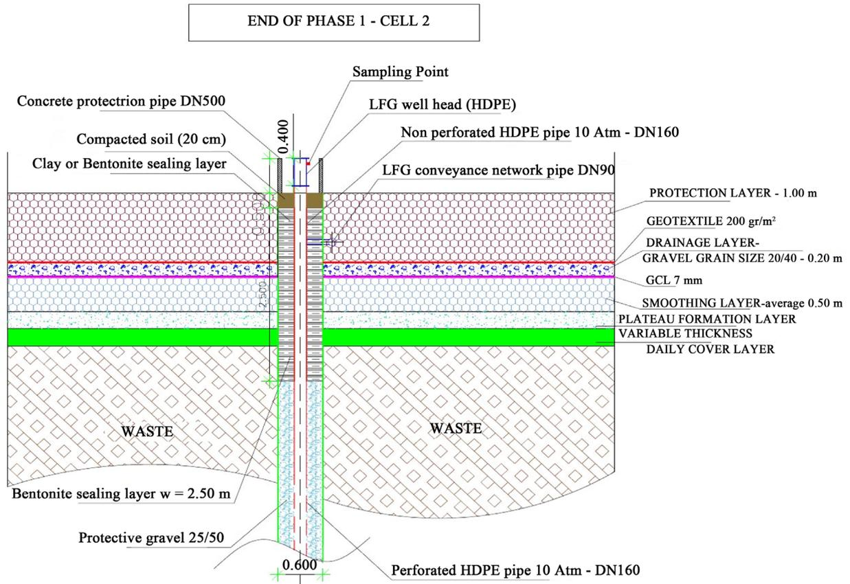
Figure 7. Parts of the well.
