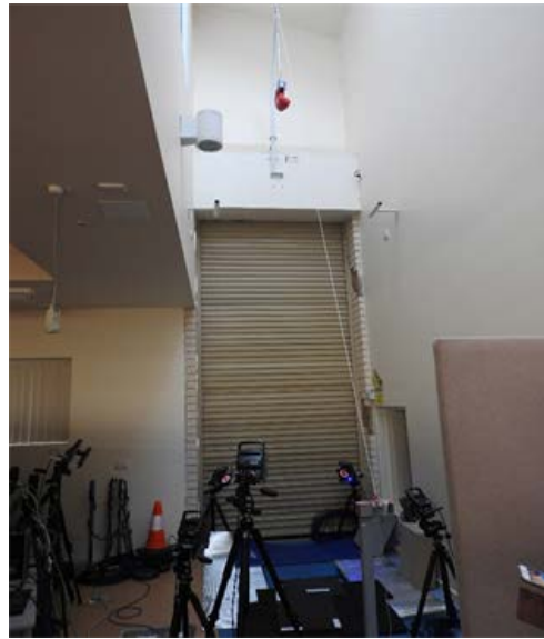
Figure 2. Drop testing system used for the experiment.
