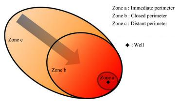
**Figure 2.** Presentation of perimeters of protection around a pumping well.
