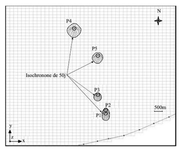
**Figure 7.** The closed protective perimeters of supply wells: 1951/27 (P1), 1950/27 (P2), 3061/27 (P3), 2024/27 (P4) and 1199/27 (P5).
