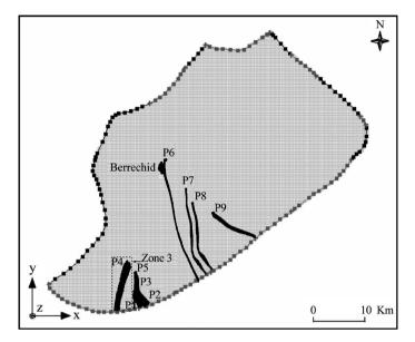
**Figure 9.** Path of water virtual particles captured by the boreholes and delimiting the protection zones.
