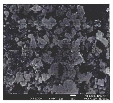
Figure 4. SEM micrograph of SnO nanoparticles.
