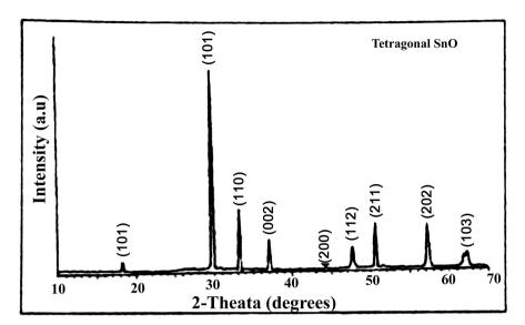
Figure 2. XRD of SnO Nanoparticles.
