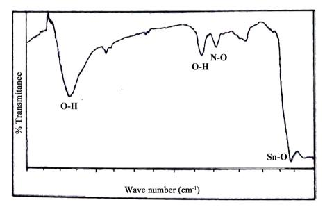
Figure 3. FT-IR spectrum of SnO nanoparticles.
