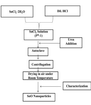
Figure 1. Flowchart for the synthesis of SnO Nanoparticles.
