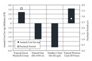
Figure 4. Effect of the CHP fuel used on the cost savings and payback period for the facility analyzed in Case 1.
