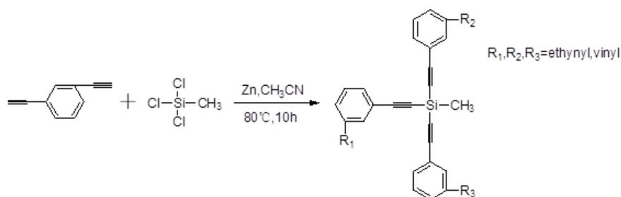
**Figure 1.** The reaction scheme of BSA resin.
