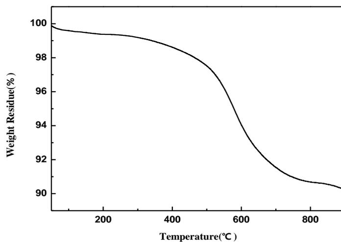
**Figure 2.** TGA curve of cured BSA resin in  $N_2$ .
