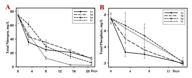
**Figure 3.** Removal of N(A) and P(B) removal from industrial wastewater by duckweeds. La: *L. aequinoctialis*, Sp: *S. polyrhiza*; Lp: *L. punctata*; Lt: *L. turionefera*.
