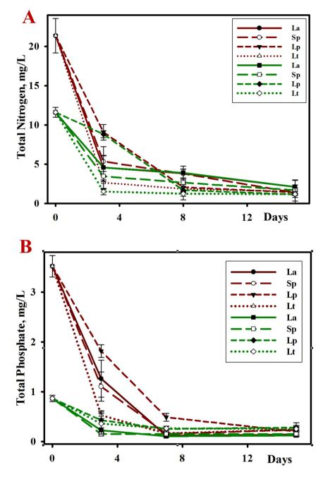
**Figure 2.** Removal of N (A) and P(B) from municipal wastewater by four duckweed species. Red lines refer to duckweeds cultivated in influent waistwater, and the green lines refer to to duckweeds cultivated in effluent wastewater. La: *L. aequinoctialis*, Sp: *S. polyrhiza*; Lp: *L. punctata*; Lt: *L. turionefera*.
