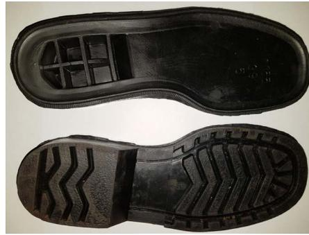
**Figure 8.** Soles produced using a composite containing 89% of products from renewable resources.
