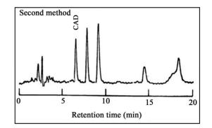
Figure 3. HPLC Chromatogram for procedure II (same as I except chloroform was used in the extraction step instead of diethyl ether) for separation of polyamines (20 minutes run).
