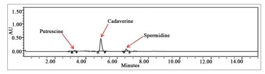
Figure 6. HPLC Chromatogram control group extracted and diluted with buffer at 1:8 ratio of polyamine:buffer (with putrescine dilution, procedure I).
