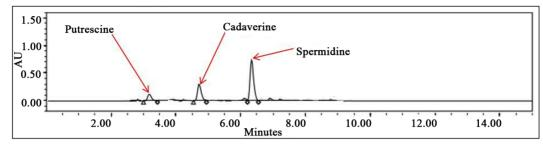
Figure 5. HPLC Chromatogram of experimental group with polyamines extracted and diluted with buffer at 1:8 ratio of polyamine:buffer (with putrescine dilution, procedure I).
