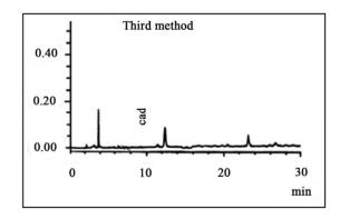
Figure 4. HPLC Chromatogram for procedure III for separation of polyamines 20 minutes run (same was I except with heated column).
